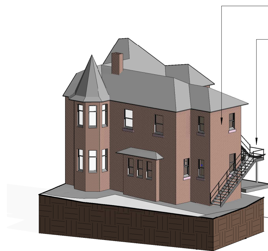
1940s BATHROOM EXTENSION TO BE DEMOLISHED EXTERNAL STAIR TO BE DEMOLISHED AND EGRESS RECONFIGURED
